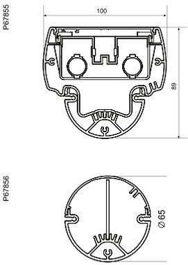
Technical drawings of the POL-OM service pole. The front view (top) shows a width of 100 mm and a height of 89 mm. The top view (bottom) shows a circular profile with a diameter of 65 mm. Reference codes P077055 and P077056 are indicated.
