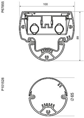
Technical drawings of the POL-O service pole. The front view (top) shows a width of 100 mm and a height of 89 mm. The top view (bottom) shows a circular profile with a diameter of 65 mm. Reference codes P077055 and P101528 are indicated.
