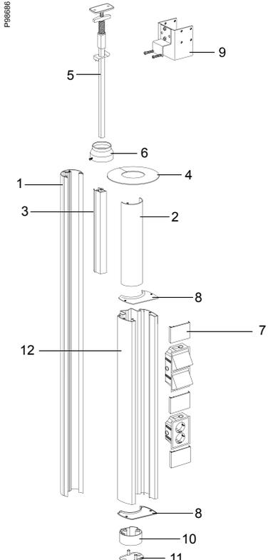
Exploded view diagram of the POL-O service pole. The diagram shows the assembly of various components, numbered 1 through 12. Reference code P066886 is shown.
