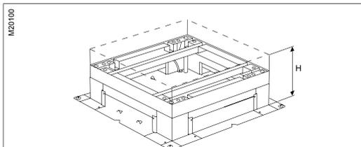
The measure H must not be smaller than the stated minimum screed depth for floor outlet boxes.
