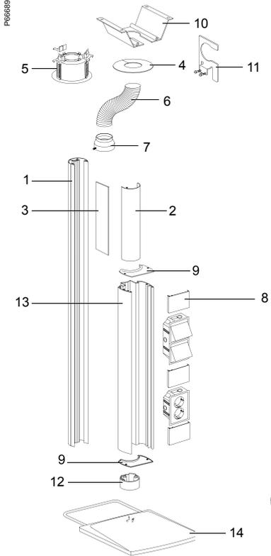
Exploded view diagram of the POL-OM service pole. The diagram shows the assembly of various components, numbered 1 through 15. Reference code P066889 is shown.
