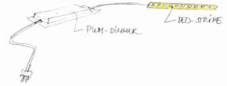
In case of larger installations to be connected to a common control, it may be more economical to look at alternative solutions. One of the alternative is common conventional power supply and several external controllers connected to it. It is an ideal choice for installations up to 10A.
