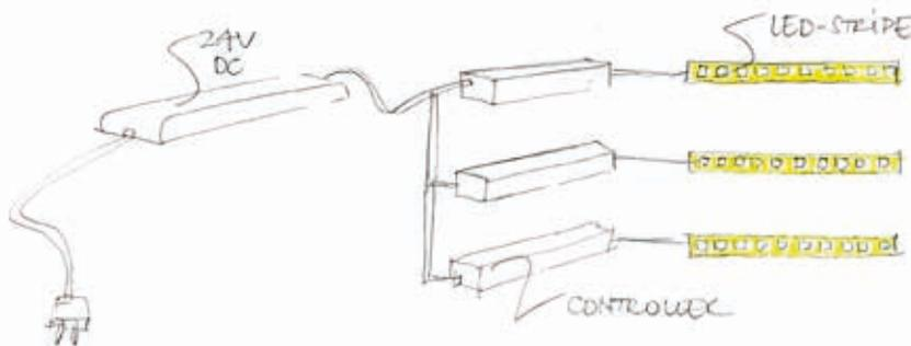
If the installation requires more than 10A, repeaters should be chosen to expand the capacity. A repeater will act as a slave module for the controller and perform the same tasks with 100% accuracy. The master controller should only control repeaters which are connected to the LED strips.
