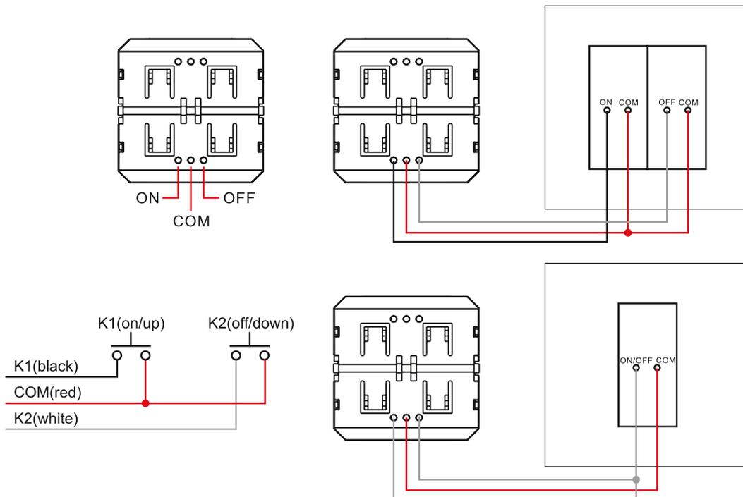
**Note :** This remote controls 1 zone (area) receivers, the zone can pair with countless receivers.
