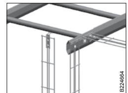
B30-I mounted onto cable ladder.
