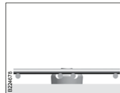
B30-I mounted onto Mounting spacer B22.
